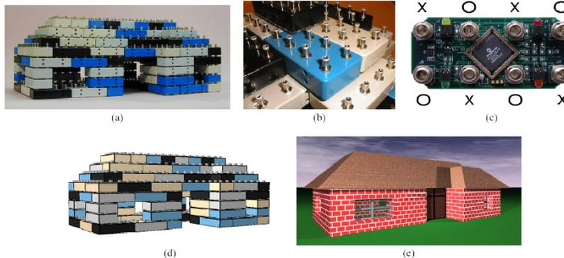
Figure 1: (a) a physical block structure comprising 98 blocks; (b) a close-up of the blocks; (c) a bottom view of the circuit board inside each block; and renderings of the virtual model recovered from the structure, one literal (d) and one interpreted (e). The literal rendering uses associated shapes and colors to render the blocks. The virtual model is augmented automatically for the interpreted rendering.
