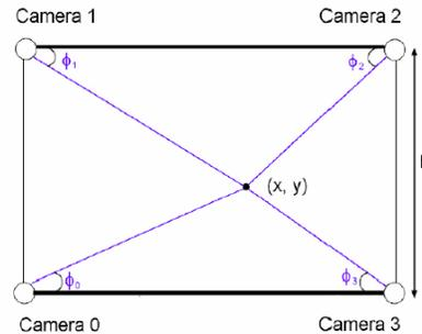
Figure 2: Camera Identification of a Contact Point
