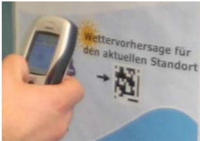
Figure 7. Taking a picture of the marker in the visual physical hyperlink interaction technique
