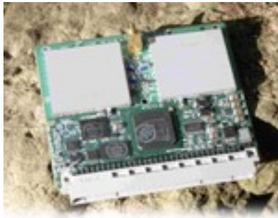
Trimble DGPS RTK Receiver Board
