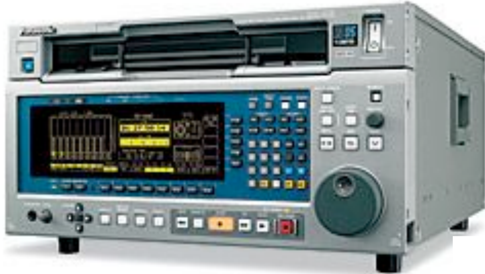
Panasonic AJ-HD3700B D-5 HD Studio Mastering System 4:2:2, 10 Bit Recording (Listenpreis $ 75,000)
