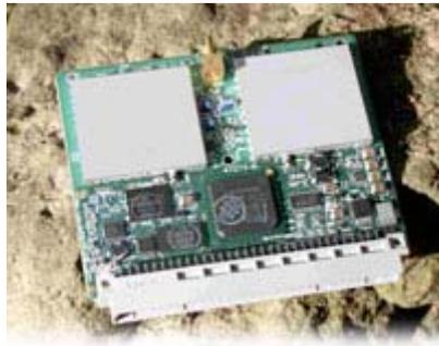
Trimble DGPS RTK Receiver Board
