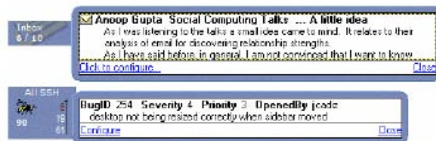
Figure 3: Two types of alert windows provided by Sideshow. When new mail arrives or when a bug of interest changes, a window fades in with a summary of the information. Users can click on the alert window to get more information.
