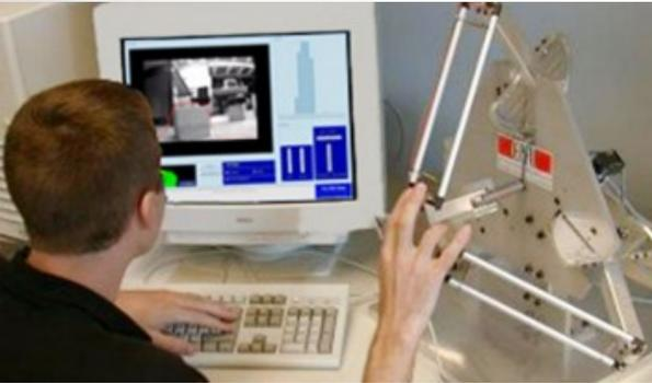
A mobile robot controlled through a haptic device.
