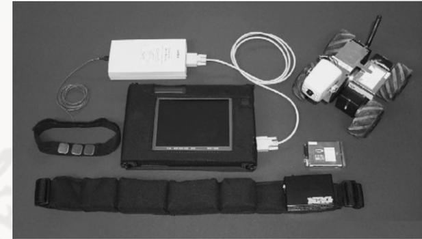
A small mobile robot controlled via brainwave.
