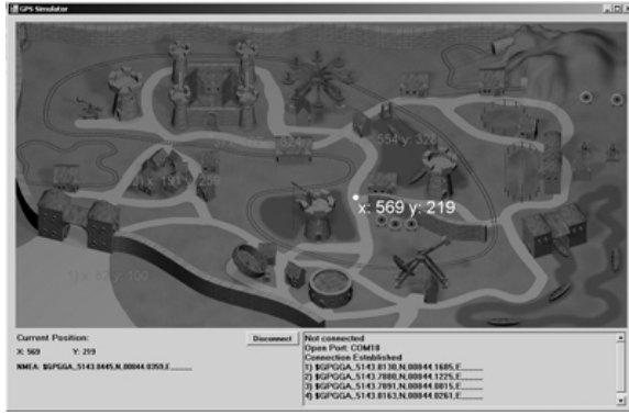
Figure 2: GPS emulator with virtual map
