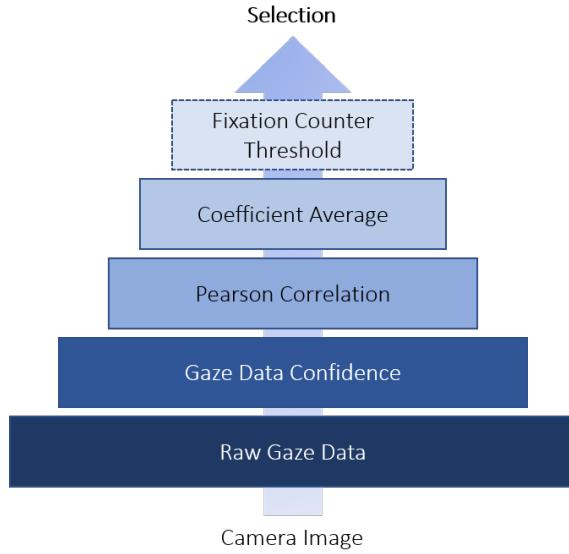
Figure 4.2: Schematic depiction of the filters the gaze data has to pass before it results in a selection. The Fixation Counter is optional.
