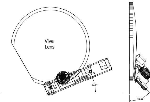
Figure 4.1: Drawing of a right lens of the HTC Vive with the Pupil Camera attached. The camera is rotated and tilted in a way that the lens can focus on the pupil of the user. For the left lens the camera is rotated by  $180^\circ$  so that the lens is at the right edge instead of the left. This also means that the two cameras have two different coordinate systems. (Picture was generated from a CAD file received from Pupil Labs)
