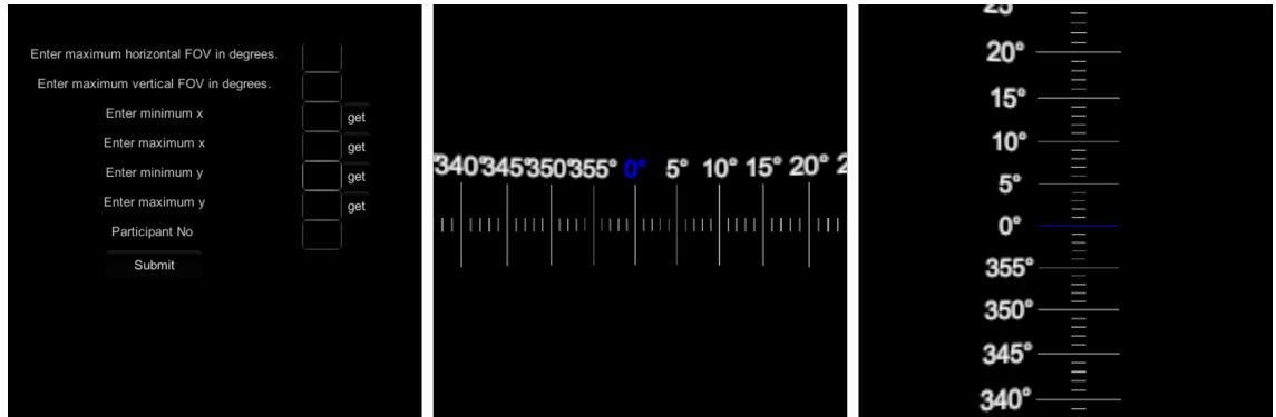
Figure 4.6: **Left:** Input form for the acquired data. The “get” buttons convert the current x- or y-position of the vertical or horizontal red line into pixels and enter the value in the corresponding box. The “submit” button writes the measurement data to a CSV file. **Middle:** Horizontal scale that was presented to the users in order to determine their horizontal FOV. **Right:** Vertical scale that was presented to the users in order to determine their vertical FOV.
