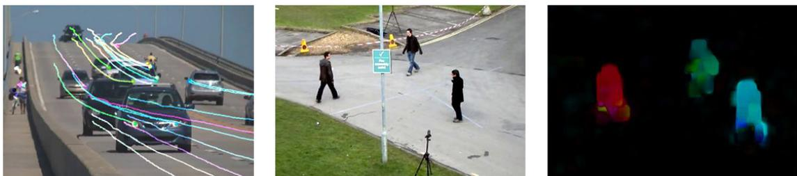
Figure 2.3: Optical flow methods<sup>1</sup>. Left: sparse flow by Lucas and Kanade [41], middle and right: dense flow by Farnebäck [25]
