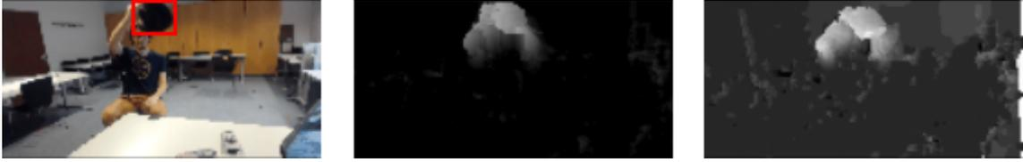
Figure 4.5: Correlation map applied to a real example. The users gaze follows the moving object indicated left. Middle: results using PCC, right: results using density method.
