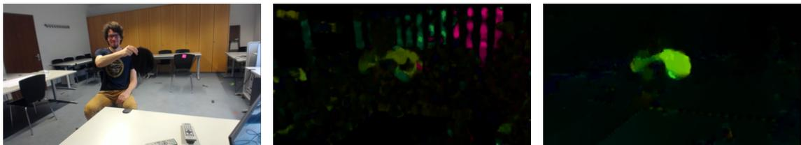
Figure 4.2: Comparison of Farnebäck [43] (middle) and Brox [9] (right) dense flow algorithms applied to an example frame (left). Colour represents movement angle and value magnitude. In comparison Brox produces a smoother and more stable result.
