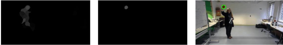
Figure 4.8: Superpixel segmentation. Mapping of correlation to superpixels (left), extraction of the strongest match (middle) and resulting object (right).
