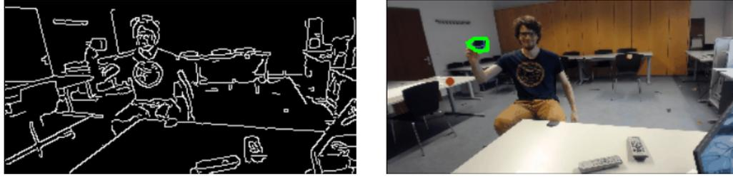
Figure 4.9: Successful object extraction with matching to "Canny-Segments". Left: edge detection with Canny, right: correct object proposal.
