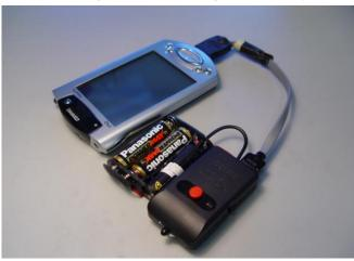
Figure 3. The components of the mobile terminal for physical browsing. The box on the right is the central SoapBox acting as the tag reader. In the battery case in the middle there is a laser pointer.
