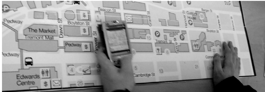
Fig. 1. RFID-only prototype permitting direct interaction with the paper map by swiping, click-selecting, and circling areas. The prototype was used to express queries such as “what restaurants are along this street?” by first constraining a query by selecting a paper menu item, and then identifying the region of interest.
