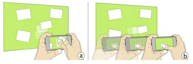
**Figure 7.2:** Moving a finger versus moving the device for dragging content. (a) Moving the finger while keeping the device steady. (b) Performing a touch-and-hold operation and moving the device with the finger remaining at its location.
