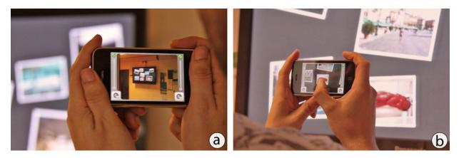
**Figure 7.7:** Walking closer to the display for higher precision. (a) A 50" screen viewed at a distance of 1.6 yards fills only 30% of the mobile display. (b) In order to see a 2" object large enough for precise manipulation, the user has to go very close to the display.
