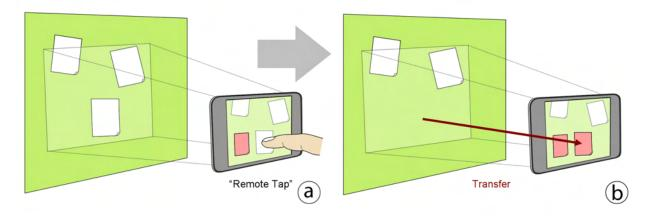
**Figure 6.11:** Transferring content to the mobile device: When the user taps a remote item (a) it is transferred to the mobile device (b). Red items denote local content.
