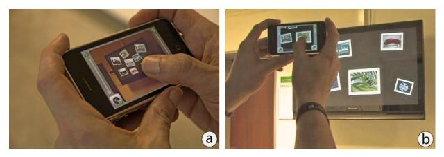
**Figure 7.10:** Freezing the live video image: (a) The live image is frozen without zoom and any further manipulation. Immediate feedback can then only be given by the target display. (b) Freezing can be combined with zoom and further be overlaid with computer-generated graphics for higher image quality and more precise interaction.
