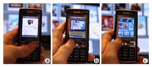
**Figure 5.7:** Connecting and selecting content *through the display*: While the application launches, the system connects to the display already with a specialized service name (a). Then the camera preview is shown which allows users to aim at content of interest (b). After capturing an image, users can decide whether this image has the content in its center (c).
