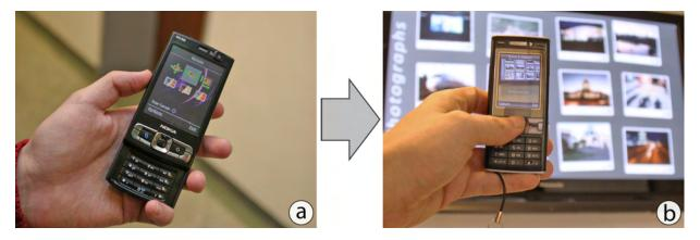
**Figure 8.2:** *Relative* versus *absolute* pointing: (a) A prototype for *relative* input showing an individual menu on the mobile device. (b) Our first system that allows for *absolute* pointing on external displays using touch input *through the display*.
