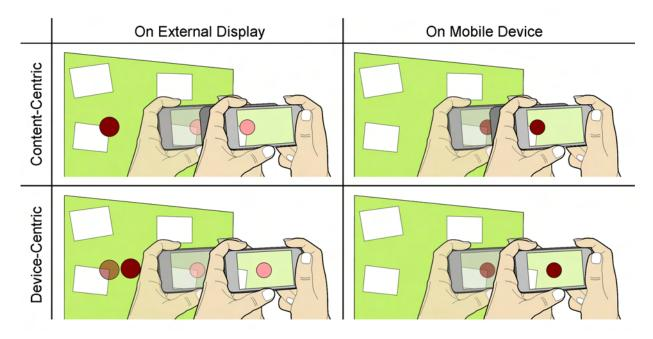
**Figure 6.6:** *Content-centric* versus *device-centric* feedback movement: The left column denotes feedback shown on the external display. In case of *device-centric* movement, the feedback item needs to move on the external screen according to the mobile device. The right column depicts the placement on the mobile device. If feedback moves in a *content-centric* way, the environment manager needs to update its position on the mobile display according to the mobile device's movement.
