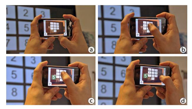
**Figure 6.12:** Showing individual feedback on the mobile device: The user points the device at the target display featuring a virtual keypad (a) and taps on a number (b). The mobile device shows the pressed number only to the respective user (c) for a certain amount of time even when the user is not tapping the number anymore (d).
