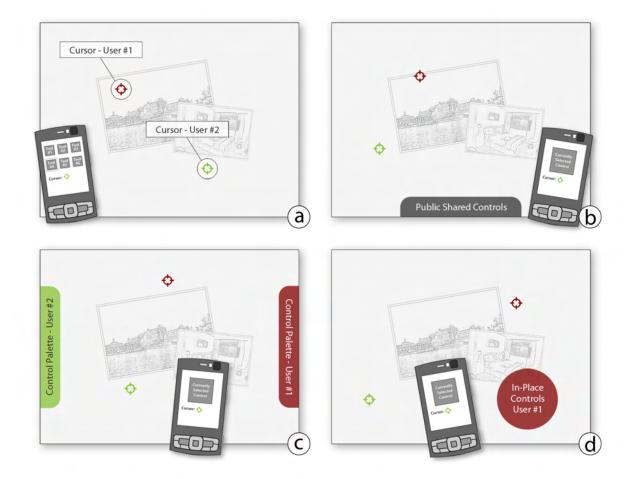
**Figure 4.9:** The four different tool palette placements: (a) depicts the *ultra-private* controls entirely displayed on the mobile device. (b) shows the *shared* tool palette accessible by every user. (c) denotes the *personal* tool palettes displayed on the public display. (d) shows a recently "called" *temporal-personal* menu (here by user #1).
