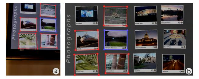
**Figure 5.5:** Matching the location of detected items (red) relative to the reference item (blue). Left shows the taken image and right shows the predicted positions based on the reference item. Although the lower right item is off by several pixel, the system can still match it according to its position. However, the detection shows errors which does not allow for taking the reference item to compute the final transformation matrix.
