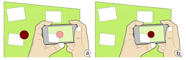
**Figure 6.5:** Placing feedback on the external display or on the mobile device: (a) The feedback is placed on the external screen and therefore also shown on the mobile display. (b) The feedback item is entirely shown on the mobile device only and does not interfere with other interactions on the external screen.
