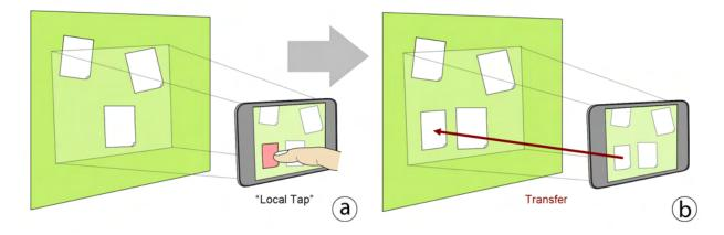
**Figure 6.10:** Transferring content to an external display: When the user taps a local item (a) it is transferred to the external display (b). Red items denote local content.
