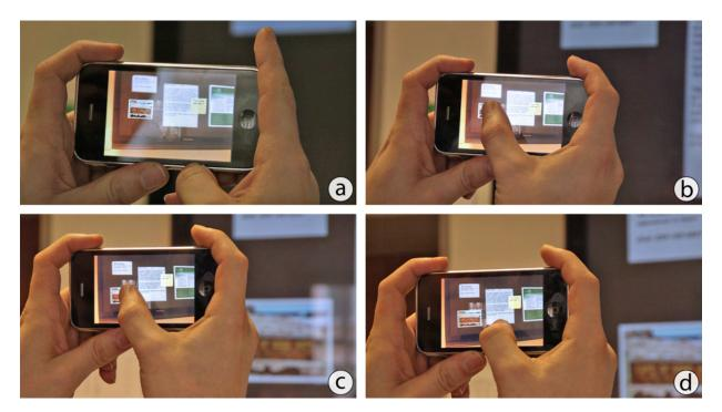
**Figure 6.13:** Transferring content from the mobile device to an external screen: The user points the device at the target display (a) and taps on a local content item (b). The tap initiates the transfer of the selected content (c) which is *moved* onto the target display (d).
