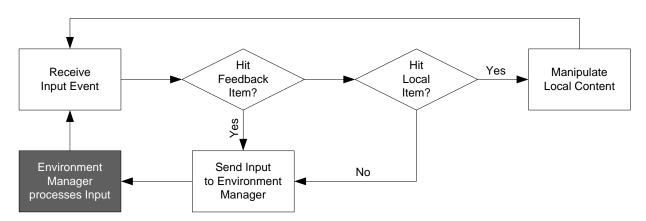
**Figure 6.9:** Input handling for local and remote content: The shaded area denotes the actions taken by the *environment manager*.
