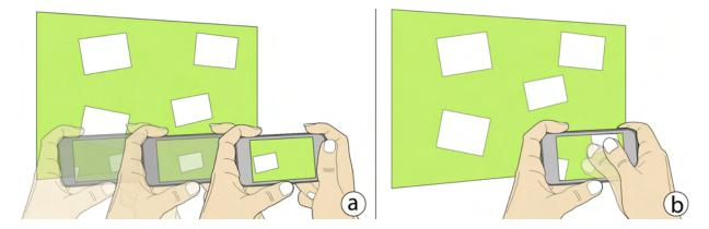
**Figure 6.1:** Coarse and fine-grained bimanual interaction. (a) Moving the device spans the reference frame. (b) A finger can then interact in this reference frame.
