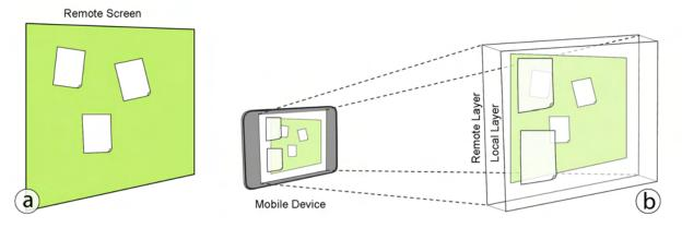
**Figure 6.4:** Two independent content layers: The external display (a) is shown in the background layer with the mobile device's content being superimposed on it (b).
