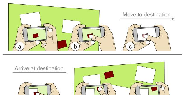
**Figure 7.4:** Dragging content across displays with the original metaphor: The user aims at a display (a) and touches the item of interest (b). When moving the device off-screen, a thumbnail of the item is shown (c). After reaching the destination display (d), the item can be positioned precisely (e). When the finger is released, the item has been transferred (f).
