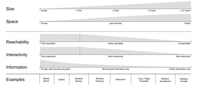
**Figure 1.2:** Dependency of display properties: if the displays' sizes increase, they are placed in public spaces. However, reachability, interactivity, and the types of information that can be used are limited more and more when displays get larger.
