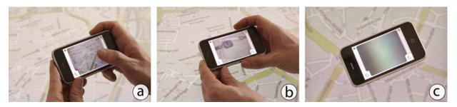
**Figure 8.6:** Problems of live video with directly superimposed displays: (a) At distances of several inches users can interact in a sharp video image. (b) Getting closer blurs the video image. (c) Placing the camera on the external screen makes the video unusable.
