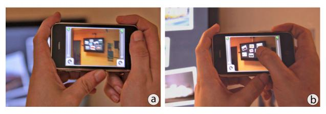
**Figure 7.6:** Two limitations of the naïve implementation: (a) Unstable images caused by the mobility of the camera in combination with slight hand movements. (b) Items are already too small for touch interaction although the display is not far away.
