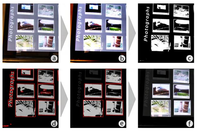
**Figure 5.1:** Preprocessing of pictures taken by a mobile device: the contrast of the original image (a) is first increased (b) for better contour detection. Thresholding the image allows removing the background (c). A blob detection finds connected components (d). These blobs are then filtered by removing too small (or too large) blobs as well as dismissing blobs that are placed entirely inside others (e). The remaining blobs are then used to "cut" the regions of the original image (f).
