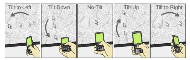
**Figure 4.4:** Controlling a pointer by tilting the mobile device: the more the device is tilted in a direction, the faster the pointer moves in this direction.
