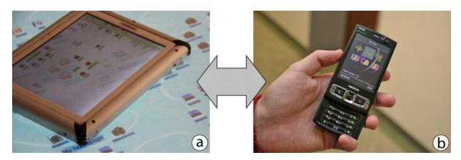
**Figure 8.1:** *Close* versus *variable* distance: (a) *LucidDisplay*, a prototype working at *limited* distances only. (b) *MobileVue*, a system allowing for interacting at *variable* distances.
