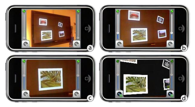
**Figure 7.13:** The four *Touch Projector* interfaces used during the study: (a) Original camera interface. (b) Manual zoom capabilities. (c) Automatic zooming. (d) Freezing the camera image with temporary overlay for precise interaction.
