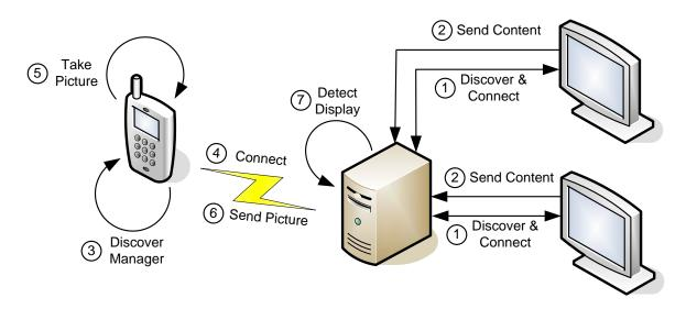
**Figure 5.12:** Architecture for environments with multiple displays: On startup, each display discovers the *environment manager* and connects to it (1). They also send their content for image analysis (2). Mobile devices also discover the environment manager (3) and connect to it (4). When users take a picture (5), the image is sent to the managing instance (6). There it is analyzed based on the content of each and every display (7).
