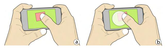
**Figure 6.8:** Distinguishing a local tap from a tap on temporary feedback: (a) The user is touching a local item. (b) The local content is superimposed with temporary feedback causing the same tap to be communicated to the environment manager for further actions.
