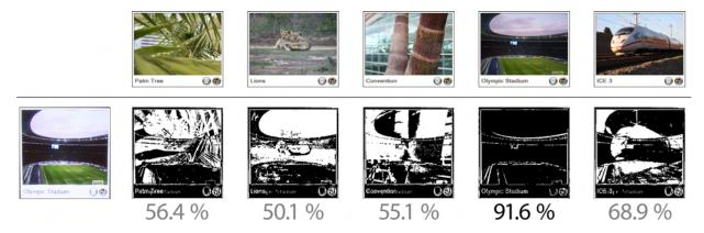
**Figure 5.4:** Similarity based on image differencing. While all images have significantly lower similarity (i.e., between 50 and 70%), the picture "Olympic Stadium" matches well with over 90%. This image is therefore the candidate for further calculations.
