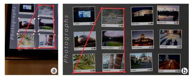
**Figure 5.6:** Optimizing the transformation matrix between mobile device and target display. Left shows the taken image and the four points producing the largest quadrangle. Right shows the four points on the target display. With this point set we achieve higher accuracy.
