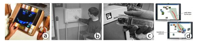
**Figure 2.16:** Transferring content across reachable devices: a) The wodden *media-Blocks* carry information [UIG98]. b) *Pick-and-Drop* uses digital pens to transfer information [Rek97]. c) *InfoPoint* embeds ea display into the pen to show carried information [KRA01]. d) *Stitching* allows content transfer through a single pen stroke [HRG<sup>+</sup>04].
