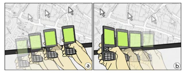
**Figure 4.5:** Moving versus tilting the mobile device: a) shows the linear mapping when the mobile device is moved. b) depicts how tilting the device increases the pointer's speed.
