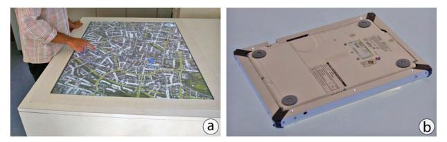
**Figure 3.6:** Devices used in our prototype: (a) Our external display is a multi-touch tabletop based on FTIR [Han05]. (b) The mobile device is embedded into a frame which contains infrared five LEDs.
