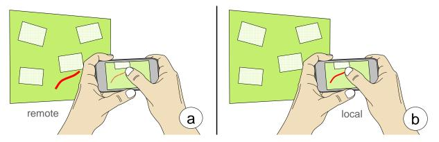
**Figure 8.8:** Rendering a line drawn either *locally* or *remotely*: (a) The line is rendered on the target display but also shown in the mobile device's viewfinder. (b) The line is drawn directly on the mobile device's screen without being shown remotely.
