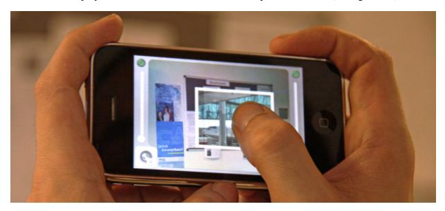
**Figure 7.3:** Visualizing dragged content in display-less space: a thumbnail is shown whenever the mobile device's camera is not pointed at a display in the environment.
