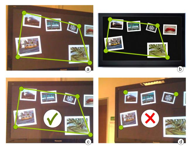
**Figure 6.2:** Feature point tracing to allow for real-time image processing: (a) The first frame is processed fully to calculate the correct transformation. (b) The corner points for the final transformation on the target display. (b) These points are found in the next frame. (c) One of the four feature points cannot be detected.
