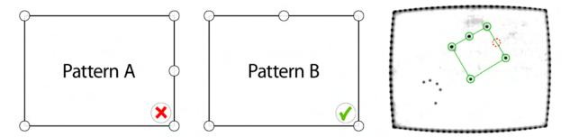
**Figure 3.7:** Different LED placements for mobile devices: Two possible patterns for LEDs on a mobile device. Right shows a sample frame from our tabletop with both a tablet PC as well as a hand being placed on it. In this scenario, pattern B can be detected.
