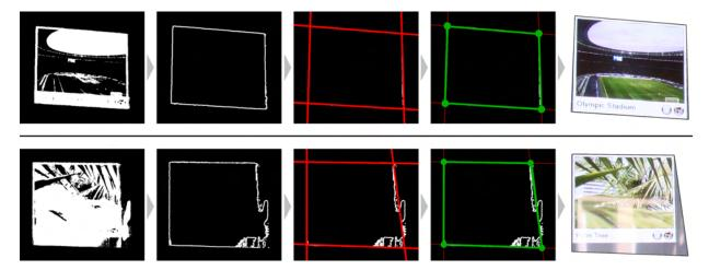
**Figure 5.2:** Detecting polygons in the captured image for a good (*top*) and bad (*bottom*) blob. From left to right: The contour of the detected blob is first calculated. A hough transform calculates lines (denoted in red). Intersecting these lines leads to a polygon (depicted in green). The polygon is used to "cut" the respective portion out of the taken image.
