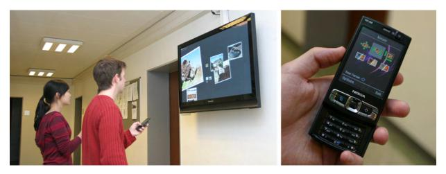
**Figure 4.12:** Two users interacting on the public display: left shows both users controlling their pointers individually. Right denotes the visual interface presented on the mobile device.
