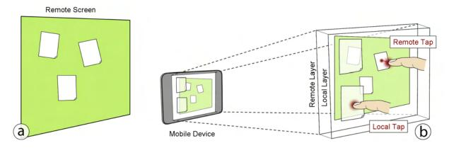
**Figure 6.7:** Distinguishing local and remote input events: When the user points the mobile device at a remote screen it shows both local and remote items (a). The items are shown on two distinct layers with the local one in the foreground and the remote one in the background (b). The received input is first processed on the local layer and then – if no item was hit – sent to the remote layer (i.e., to the remote screen) for further input handling.
