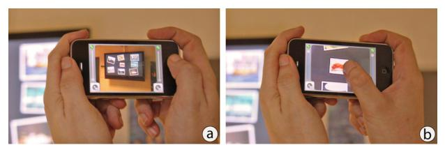
**Figure 7.9:** Zooming automatically based on the display's distance: (a) The display's size in the viewfinder does not allow for precise interaction. (b) To allow a constant CD ratio across all displays, the system zooms into the video image automatically based on the display's distance and size. The zoom factor is updated permanently.
