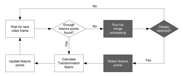
**Figure 6.3:** The image recognition process for real-time feedback. The shaded areas denote the processes with high computational requirements. These can be left out as long as feature points are available and can further be detected in the new frame.
