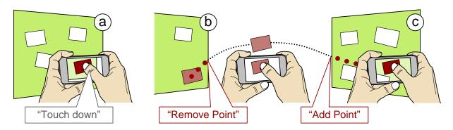
**Figure 7.5:** Touch event handling when interacting across displays: (a) A touch event is projected onto the current screen. (b) Leaving the screen requires a removal of the point. (c) Reaching another screen then requires the manager to add a new touch point to the display.
