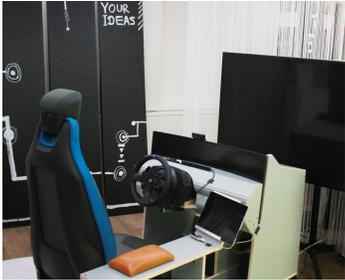
**Figure 1:** The seating box combines a driving simulation with sensors (gaze, gestures, video) and a versatile combination of touch and ultra wide screen display to allow prototyping for future IVIS.
