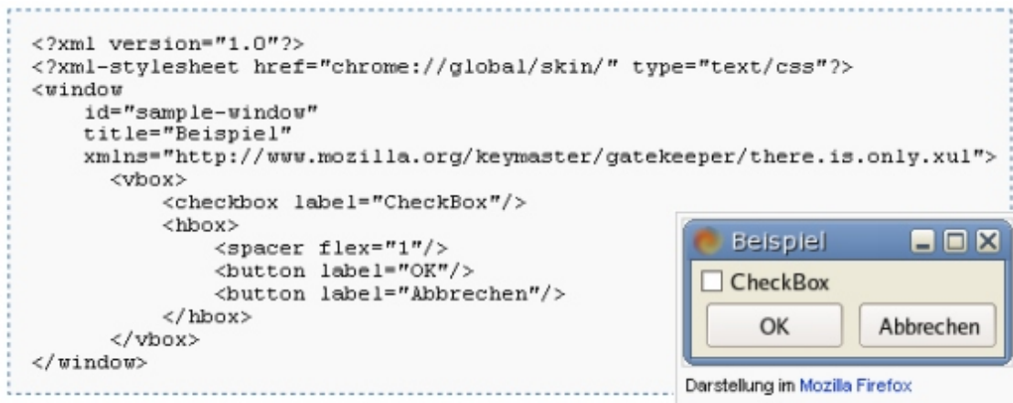
Figure 2.4: Example of XUL code and the rendered interface (from [wiki a])
