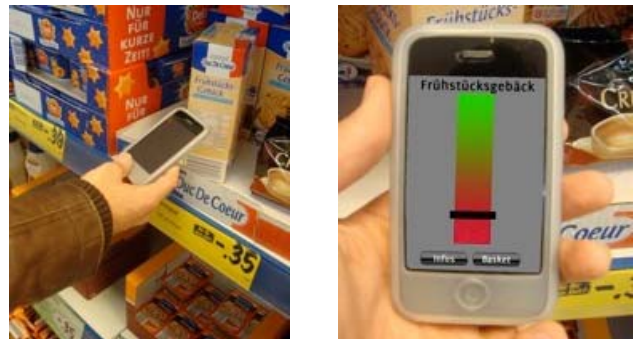
Fig. 1. Mockup of a diabetes shopping assistant revealing the amount of sugar in NFC-tagged grocery products
