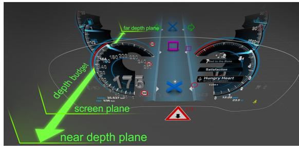
**Figure 2:** Top view of the implemented concept depicting the spatial arrangement of the displayed IC elements.
