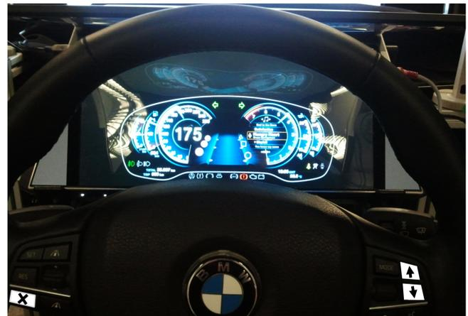
**Figure 4:** A button 'X' on the left side of the steering wheel needs to be pressed for judging the symbol's position. A toggle button ('↑' or '↓') on the right side of the steering wheel decodes the reaction on unexpected events.
