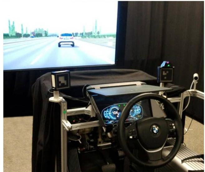
**Figure 1:** Setup of our experiment: We use a driving simulator to evaluate the influence of visualization, technology, and interface complexity on user performance and subjective perception of S3D user interfaces.
