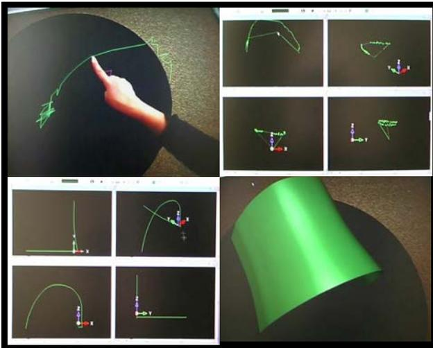
**Figure 6. 3D finger tip tracking used for shape creation within a CAD tool**
