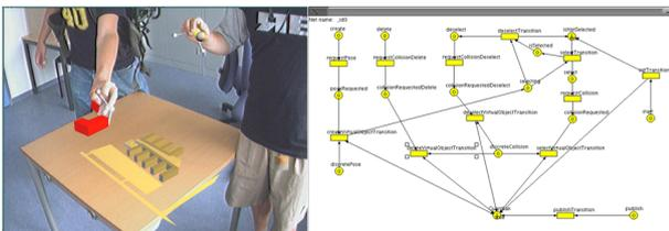
**Figure 3: Complex interactions within a tangible modelling application for architects. The corresponding Petri Net is shown on the right.**
