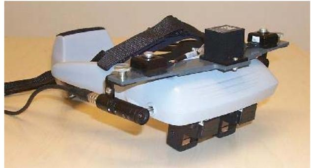
**Figure 4. Head mounted display with cameras and head tracking system. First prototype.**
