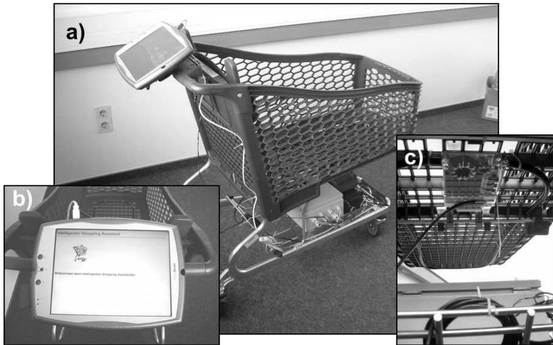
**Figure 2: Instrumented Shopping Cart (a) with Tablet PC on the handle (b) and RFID antenna on the bottom side of the basket (c).**
