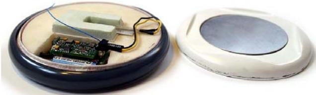
The device weighs 110 grams and works several hours on a single battery charge. Hardware cost is currently about 100 US\$ per device, but can be expected to go down below \$10 in larger quantities. Batteries can currently be charged only after disassembling the device, but this can be solved by inductive transmission through the plastic case when the mat is stored over night.
