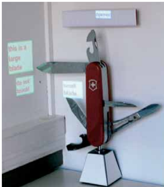
5 The object-annotation application. The application labels a complex object's subparts and projects labels where they will be easily readable.
