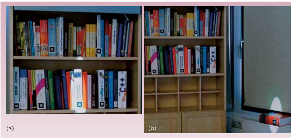
3 The SearchLight application. The system responds to query results by projecting a bright spot around the corresponding objects in the physical environment. (a) It finds one book on the shelf and (b) another lying on the windowsill.
