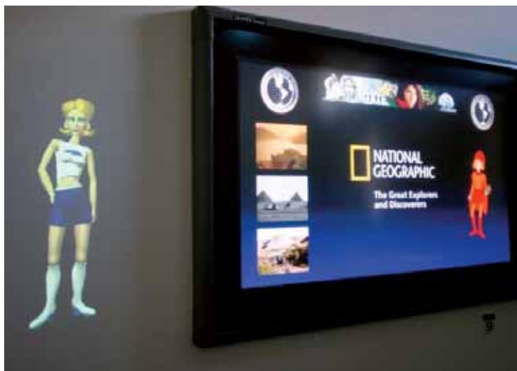
6 The virtual room inhabitant. The steerable projector projects the VRI on the wall next to a large plasma screen
