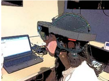
Figure 1: In this picture, the HoloLens is combined with the g.tec BCI. The Processing of the brain signal is done on the Laptop in the Background. Transmitting the HoloLens input is done with UDP.
