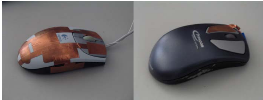
Fig. 1. The pictures show the first and second prototype of the touch-sensitive mouse.
