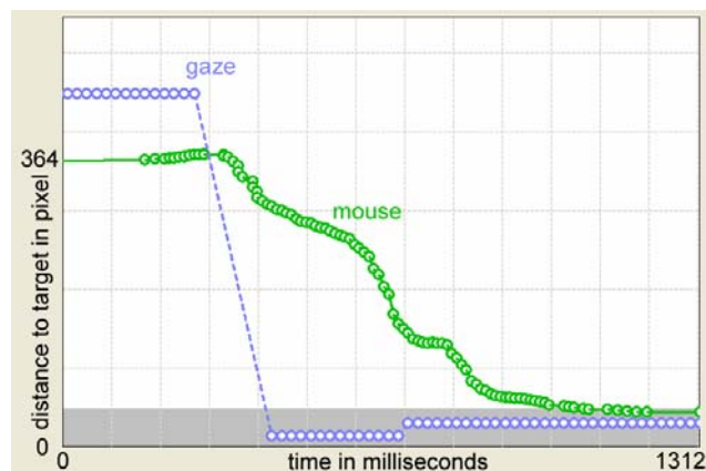
Fig. 7. Gaze (dashed) and mouse trail (solid) for the classical mouse task without background as a plot of distance to target over time.
