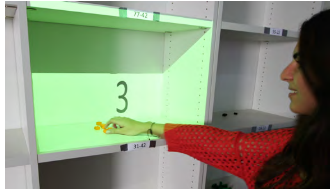
Figure 1. A participant is picking items from a shelf. The projector cart highlights the correct box and provides in-situ information about how many items to pick.
