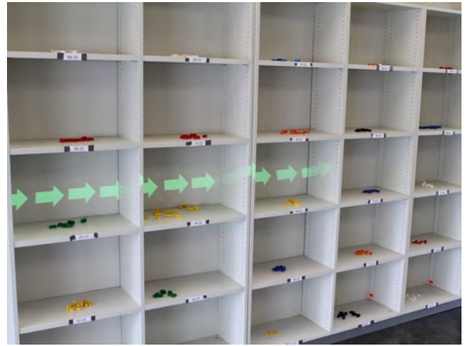
Figure 3. Arrows that are projected when the target compartment is not in the projector's field of view. The arrows are moving together with the cart and showing the shortest path to the target compartment.
