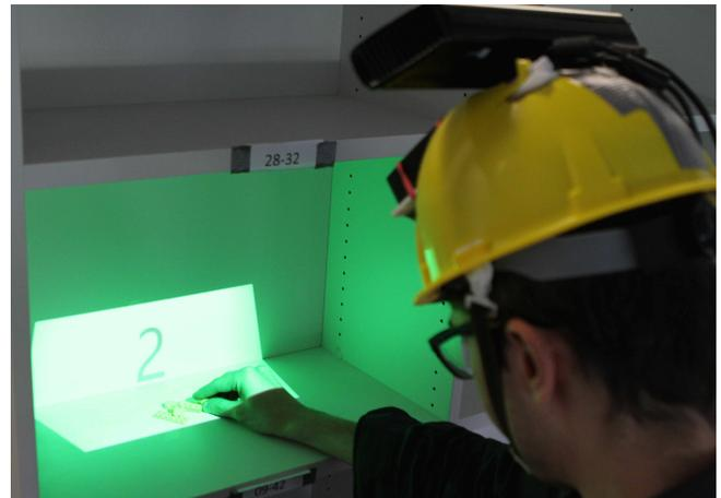
Figure 1. A user is interacting with the order picking helmet. The helmet highlights the compartments storing the items to pick and directly projects the amount of items to pick into the environment.
