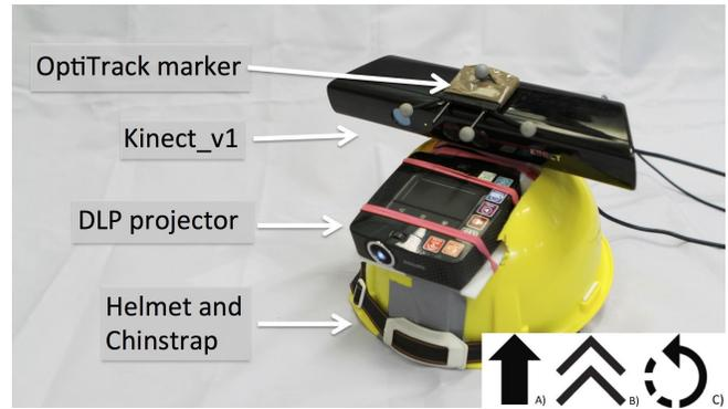
Figure 2. The HelmetPickAR order picking helmet and the arrows that can be displayed to navigate the participant.
