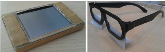
Fig. 2. Cardboard overlay to simulate different input touch areas on the iPod Touch (left) and paper blinders taped to plastic glasses to prevent peripheral view (right) [7].
