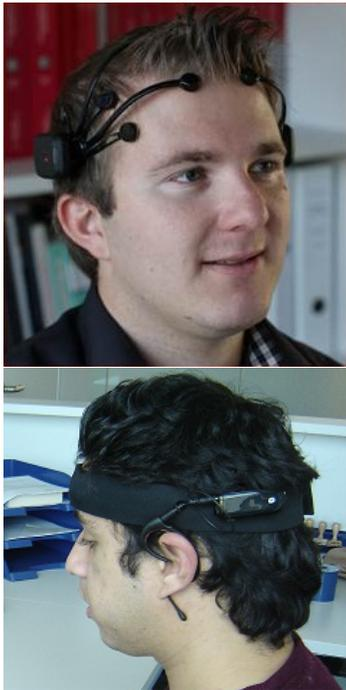
**Figure 1:** Examples of consumer BCI: the Emotiv EPOC and the Myndplay Mindband.
