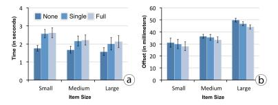
**Fig. 8.** Results of the targeting study: (a) retrieval time for one item for all feedback conditions and item sizes; (b) offset for correct retrievals measured as Euclidean distance between the item's center and the touch's location. Error bars represent 95% confidence intervals.
