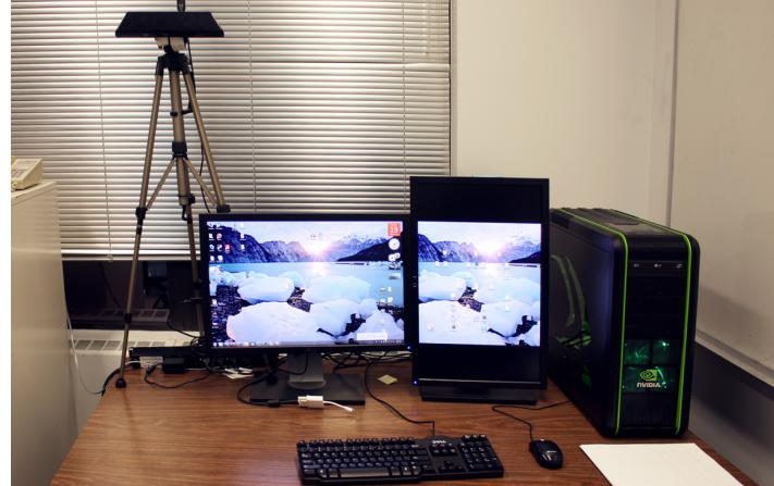
**Figure 8.4:** Setup of the Unadorned Desk 2D with the interaction area on the left of the keyboard observed by a Kinect depth camera, which is mounted facing upside down.
