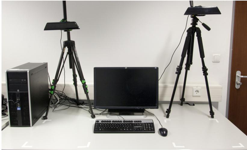
**Figure 8.13:** Study setup for the Unadorned Desk 3D with two Microsoft Kinect cameras. The interaction volume is marked on the desk to give participants some landmarks on the otherwise empty desk. Vertically, the height of the monitor was indicating the limits of the interaction volume.
