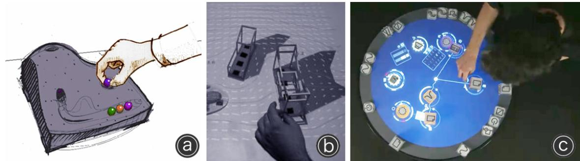
**Figure 3.2:** Examples for Tangible User Interfaces: (a) One of the very first examples, the *Marble Answering Machine* [33]; (b) *Urp*: an urban planning tool [236] from research in 1999; and (c) the *reactable* [137], a research project that was turned into a commercial product.
