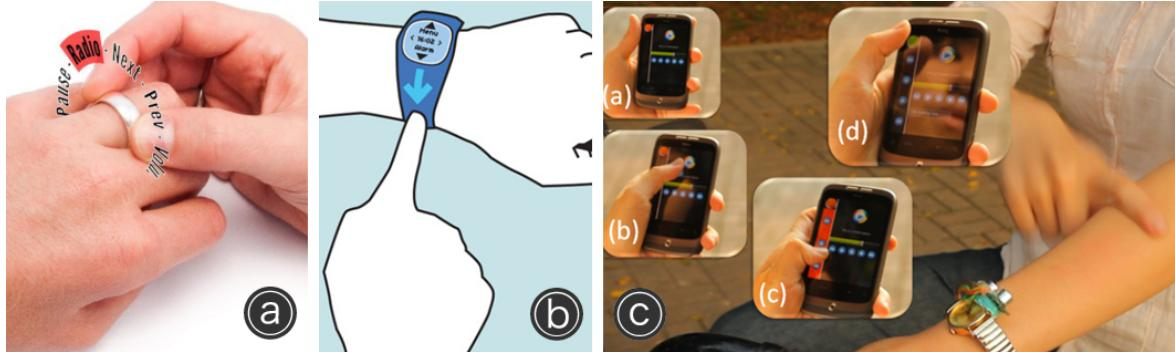
**Figure 4.1:** Example applications for eyes-free interaction: (a) the magnetic ring Nenya [12]; (b) WatchIt [192], an interactive wristband attached to a watch; and (c) Point Upon Body (PUB) [155] to control a mobile device.
