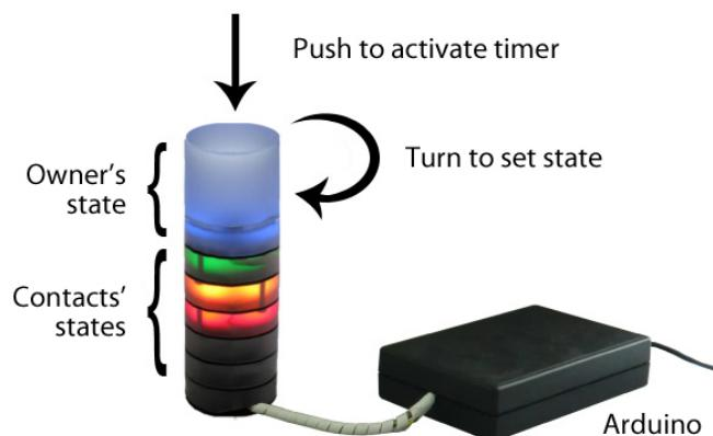
**Figure 6.4:** The prototype of StaTube. The upmost level represents the owner's state while the lower levels represent the contacts' states. By pushing down the upmost level a timer is set. By turning the upmost level the state can be changed. The black box carries the Arduino, which controls the prototype.
