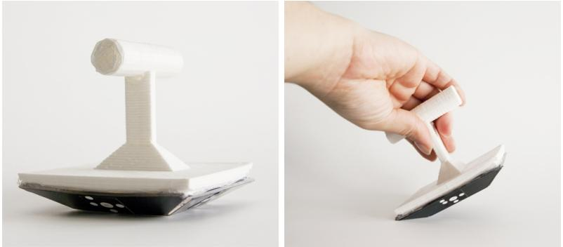
**Figure 7.11:** Graspable/Tilttable device printed on a 3D printer and equipped with markers. After tilting it, the device returns to its initial position on its own.
