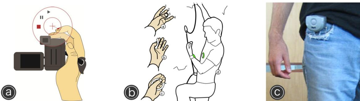
**Figure 4.2:** Example applications for microinteractions: (a) *Tickle* [263], investigating microinteractions on different shaped surfaces; (b) *PinchWatch* [156], enabling microgestures during rock climbing; and (c) *Whack Gestures* [125], interacting with a device by stroking it.
