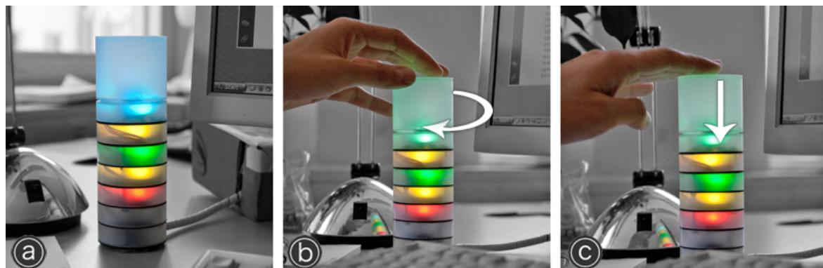
**Figure 6.1:** StaTube is a graspable device on the user’s desk. The upmost level represents the user’s own state while the other levels show selected contacts (a). By turning the upmost level the state can be changed (b). Pushing down the upmost level activates a timer (c).
