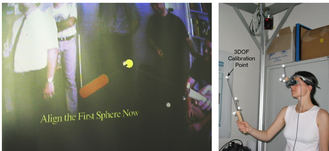
Figure 3.7: HMD calibration with a pointing device
