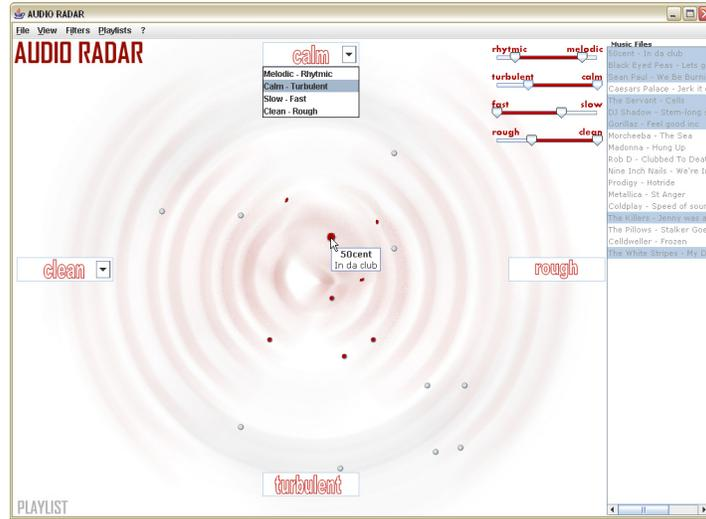
**Fig. 4.** The AudioRadar playlist creator. A red dot indicates that a song is within the currently selected attribute range while a grey dot signifies that it is excluded from the playlist. Four sliders with two thumbs on the upper right corner of the view control the ranges of the attributes. The list view on the right is linked to the radar view and selected songs are highlighted.
