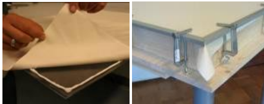
Figure 3: Building steps. Left: pouring an even distribution of the black liquid onto the acrylic and placing the latex sheet on top. Right: sealing panel with aluminum frame and silicon sealant.
