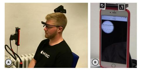
**Figure 2.** The figure shows the usability study's setup. The iPhone was mounted on a holder such that it was 30 cm away from the user's eyes (**A**). From the user's perspective, they could see the phone with the spot moving according to the user's gaze (**B**).
