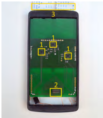
Figure 9: Case of the prototype holding a custom PCB comprising three MPR 121 (1), connectors for touchscreens (2), and flex cables (3) leading to the hardware box.
