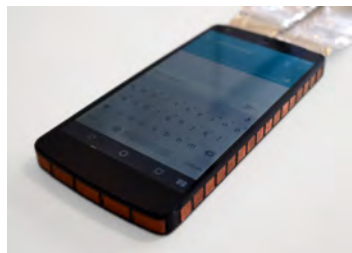
Figure 7: The full-touch smartphone prototype with touch sensing capabilities on the front, back, left, right and bottom side.
