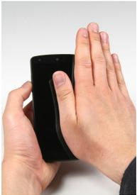
**Figure 2:** *PalmTouch* with the flat hand during two-handed use.
