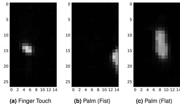
**Figure 4:** Exemplary raw capacitive images from the data collection study. Figure (a) shows the finger of participant 5 during the dragging task; (b) shows the palm of participant 19 in the one-handed condition and (c) shows the palm of participant 9 in the two-handed condition.
