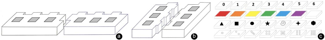
**Figure 1: MemorINO boards and cards: a) Connect horizontally, b) Connect vertically, and c) Tangible cards with images on both sides.**
