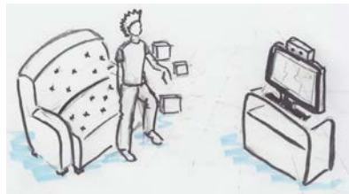
Figure 1: Overview of our concept. A user is able to control the smart home environment by placing parts of the user's body into trigger areas to trigger actions such as changing the TV channel.
