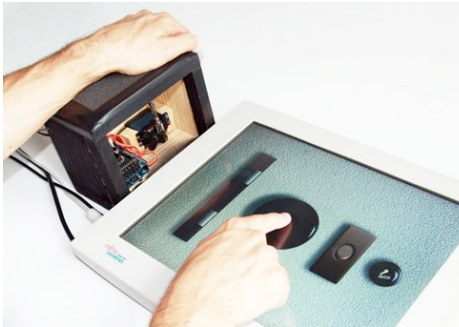
Figure 1: Implementation of our approach to recreate the input and output characteristics of mechanical push buttons on touch surfaces using a remote tactile interface.
