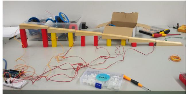
**Figure 1: MarbleTrack consists of a set of typical as well as prepared marble track elements. The prepared elements trigger sounds if the marble passes. Children can restructure melodic and rhythmic information by rebuilding the track.**
