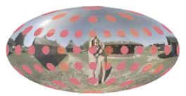
Figure 13: Hammer projection, with overlays according to Tissot's indicatrix. It has the advantage of less distortion in the pole regions, but the disadvantage of more distortion on the sides.
