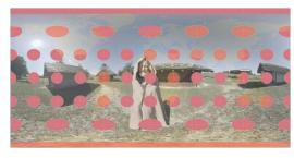
Figure 15: Equirectangular projecting, with overlays according to Tissot's indicatrix. It has the advantage of less distortion in the area around the 0°-horizontal-line, but the disadvantage of more distortion near the poles.
