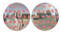
Figure 14: Azimuthal equidistant projection with overlays according to Tissot's indicatrix. It has the advantage of less distortion, but the disadvantage of a split display.
