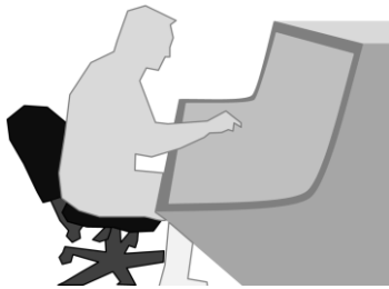
Figure 3: Curve is a non-flat display working environment designed to ease the transition between different subareas.
