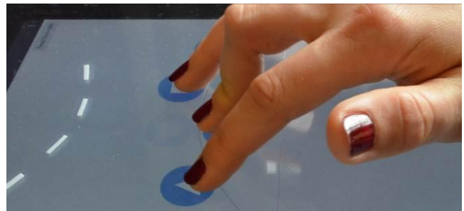
Figure 1. A silicon foil attached to a tablet forms a haptic border for guidance. It supports dragging gestures for item selection.
