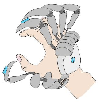
Figure 1. Outline of the Dexmo glove and the attached IMUs (blue).
