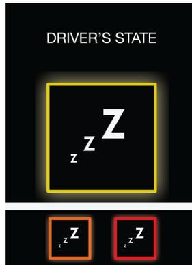
**Figure 1:** An *on-time warning* is displayed when a critical value is reached (here: drowsiness). A warning features a color-coded frame indicating the urgency.
