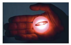
**Figure 1.** The physical interface from *Solofind* as experience prototype, equipped with a hi-power light emitting (LED) diode and a Near Field Communication (NFC) tag.
