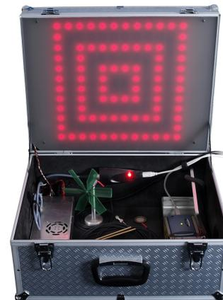
**Figure 7. The hardware prototyping toolkit LightBox, for exploring content for low-resolution Media Architecture before the final implementation [28].**
