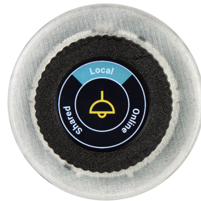
Figure 7: A close-up of a proxy interface with the three privacy states: Local, Online, and Online-Shared. Users can switch between privacy states by turning the black ring.
