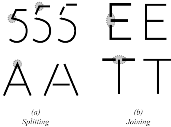
Figure 3: To create a one-to-one correspondence between strokes, the strokes of a character may be (a) split at the sharpest bend, or (b) joined where they are most nearly collinear.
