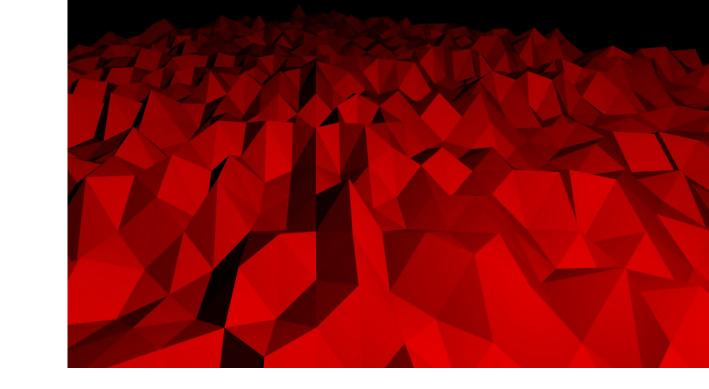
const g = new PlaneGeometry(params.size, params.size, params.fragment, params.fragment) const plane = new Mesh(g, new MeshStandardMaterial({flatShading: true, side: DoubleSide})) plane.rotateX(Math.PI/2)
