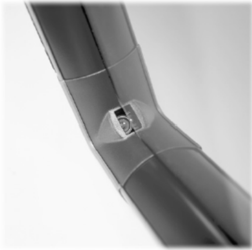
Figure 1: DViT Technology Camera
