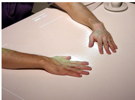
Figure 3: Interactive table with an 8 × 9 SmartSkin sensor: A sheet of plywood covers the antennas. The white squares are spacers to protect the wires from the weight of the plywood cover.
