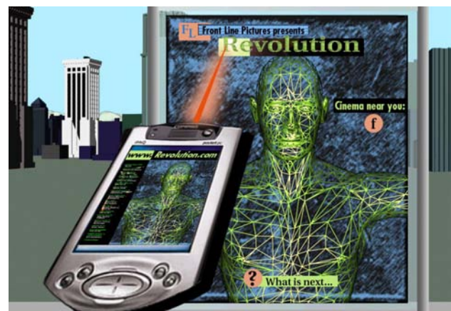
Figure 1. The user selects a link in a movie poster by pointing to it. The mobile terminal reads the tag and the web page of the movie is opened.
