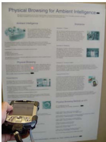
Figure 4. Physical browsing prototype being used for browsing a poster.
