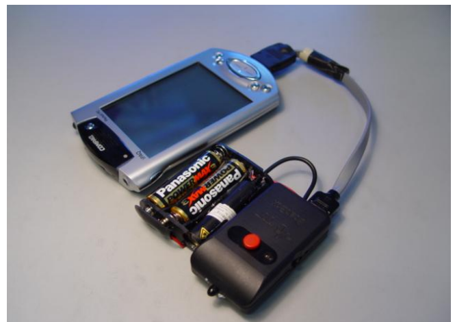
Figure 3. The components of the mobile terminal for physical browsing. The box on the right is the central SoapBox acting as the tag reader. In the battery case in the middle there is a laser pointer.
