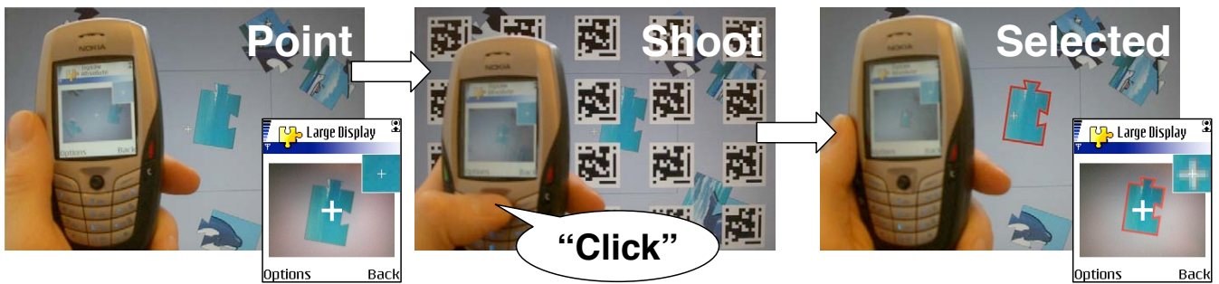
Figure 1: Point & shoot interaction: The left screenshot shows the phone screen as the user is aiming at the highlighted target. The cursor on the phone is active and the locus of attention and the cursor on the display is inactive. Pushing the joystick to the left indicates a selection at the location of the cursor on the phone display. Then the visual code grid is briefly displayed for computing the target coordinates as shown in the middle screenshot. The grid disappears again and a mouse selection occurs in the target region.
