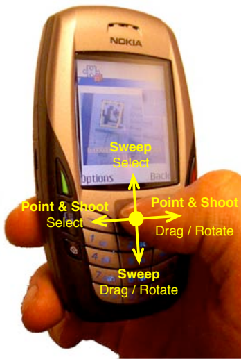
Figure 4: Phone input interaction: point & shoot is mapped to horizontal joystick push-and-release, sweep is mapped to vertical push-and-hold.
