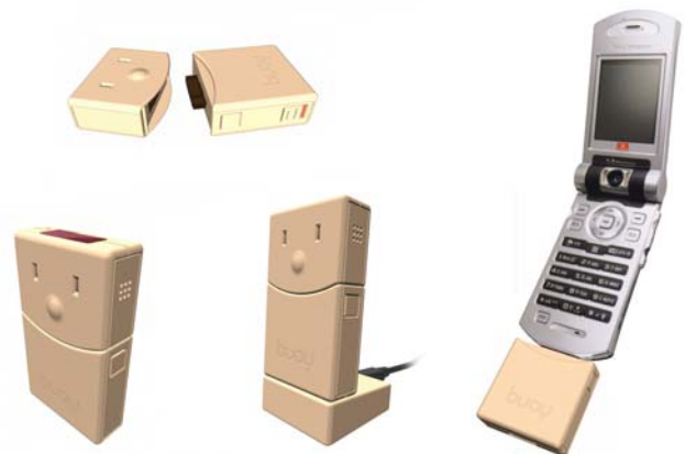
Fig 1: Three variations of the wireless discovery device: the wireless device with an add-on component, a cellular phone and cradle
